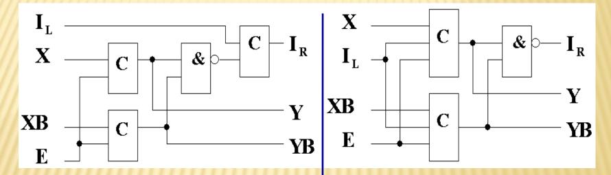
I<sub>L</sub> delay is bigger than others input delays
